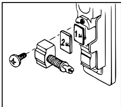
Use the correct spacers 1 & 2 to ensure the correct fit on any profiles depending on their width.
