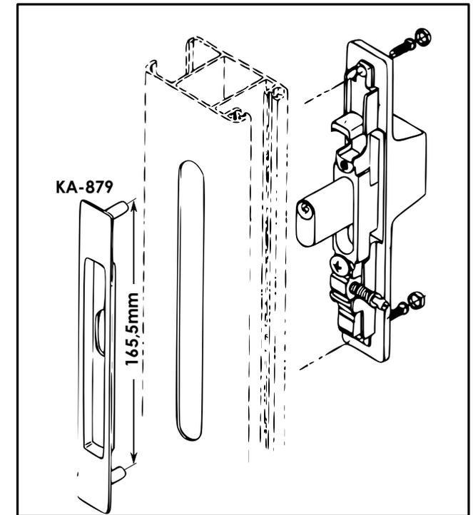
Additionally, you can fit the KA-879 opposite plate of the KA-370 & 380 instead of the locking cylinder rosette or in case you want to replace an old locking handle.
