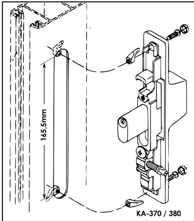
Create a hole, only on the internal face of the profile. Restraint the lock with the especially casted (hooks) components.
